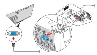
Connect one end to the projector's Computer1 or Computer2 port, and the other end to your computer's | monitor port. If you are using a laptop, switch it to external display. You can also connect an audio cable or microphone.
